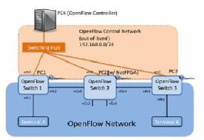
Figure 5. Generic OpenFlow network: controller and Openflow switches [9]
