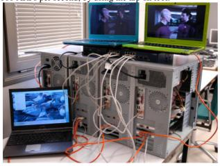
Figure 8. OpenFlow/NetFPGAs network set up
