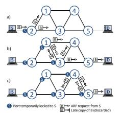
Figure 1. ARP-Path discovery from host S to host D. The small bubbles on the links show which switch port locked S's address.
