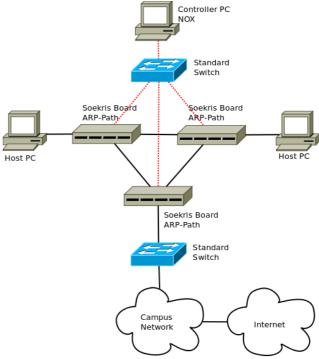
Figure 9. Test network for OpenFlow/Soekris 100 Mbps
