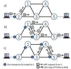
Figure 1: ARP-Path discovery from host *S* to host *D*. The small bubbles on the links show which bridge port locked *S*'s address
